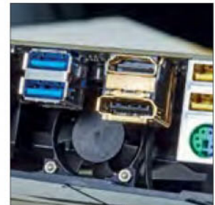
There's a small 6,000RPM fan under the I/O cover for cooling the VRM components.
