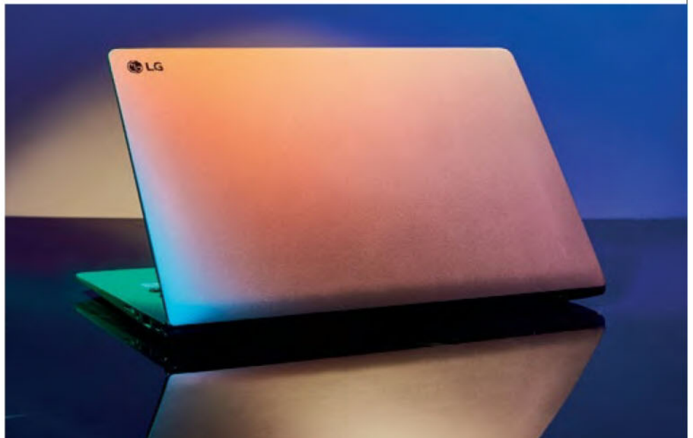
The Gram 14 is one of the notebooks to use magnesium alloy in its construction.
