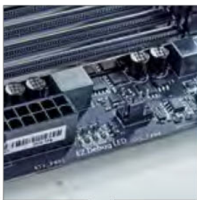
The EZ Debug LEDs stand in for a debug display in pinpointing hardware issues.
