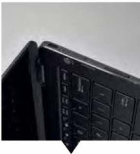
There's a fingerprint sensor hidden to the side of the ZenBook Flip S.
