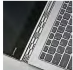
The watchband hinge allows the display to fold almost completely flat against itself.
