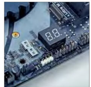
A debug LED display helps with troubleshooting.
